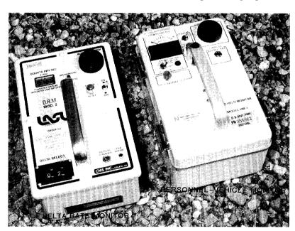
instrument more commonly used at search stations. The Delta Rate Monitor is a more specialized instrument for stations where the radiation intensity is highly variable. A thumbwheel switch on the Delta Rate Monitor allows the operator to compensate for these changes in intensity.
