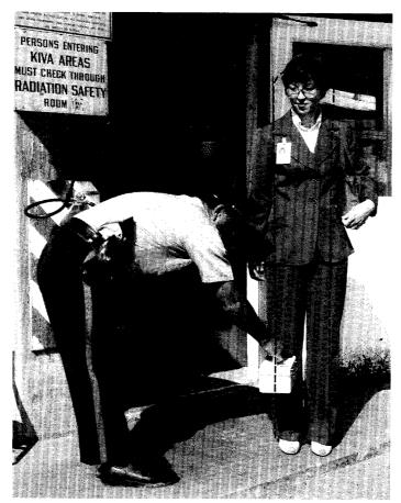
A good place to begin your scan is near one foot. Scan up one side of the body to the head, then scan down the other side. Ask the person to turn around and repeat the inverted U-shaped sweep. Pace your scan. Each sweep from head to foot should take 2 or 3 seconds. Hence, a front scan will take 5 or 6 seconds, turning around takes a few more seconds, and a back scan takes 5 or 6 seconds, for a total of 15 seconds.
